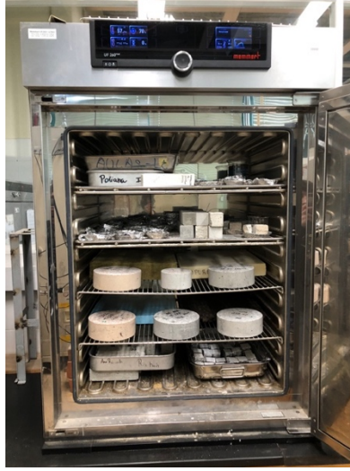
Fig. 2. Concrete samples undergoing oven drying at 60 \pm 5^\circ\text{C} until achieving constant mass, in accordance with ISO 12571 [21].
