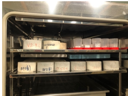
Fig. 3. Samples placed in a climatic chamber at 23 \pm 0.5^\circ\text{C} and exposed to different relative humidity setpoints for sorption curve measurements.
