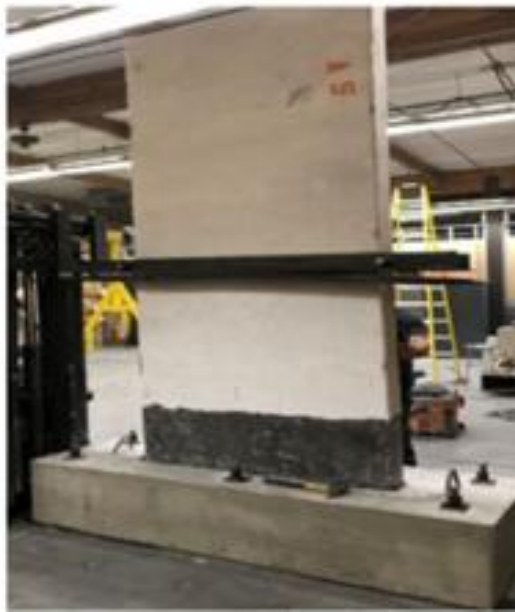
Figure 19 Integration of MSCIP wall specimen into a socket connection: socket footing wall connection (Figure adapted from [29])
