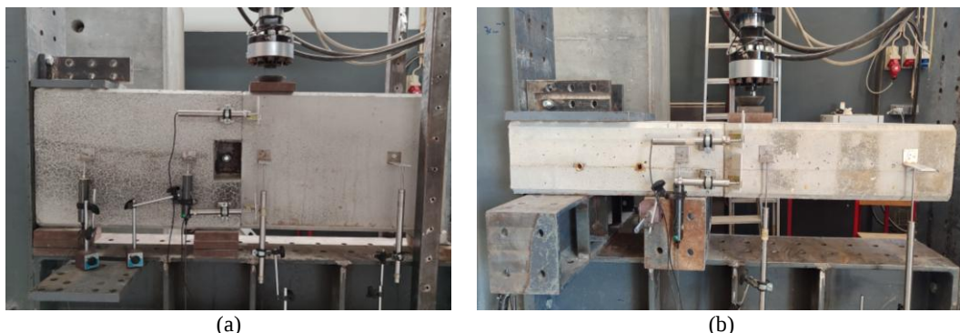
Fig. 4 Monotonic shear test: (a) In-plane of the wall; (b) Out-of-plane of the wall.
